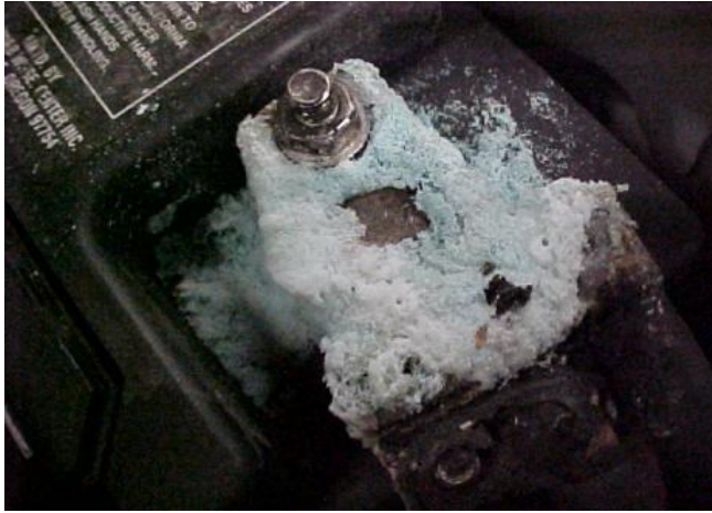
Figure 2: Corrosion on a battery may look something like this
